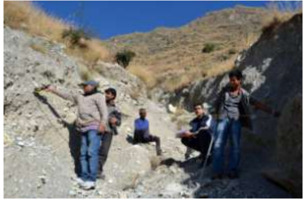
Photo 4: Measuring the width of the Gully erosion
